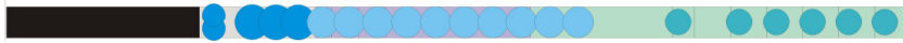
Figure 2. Nozzle distribution for circular nozzles. The nozzle areas below the mould are overlapping
