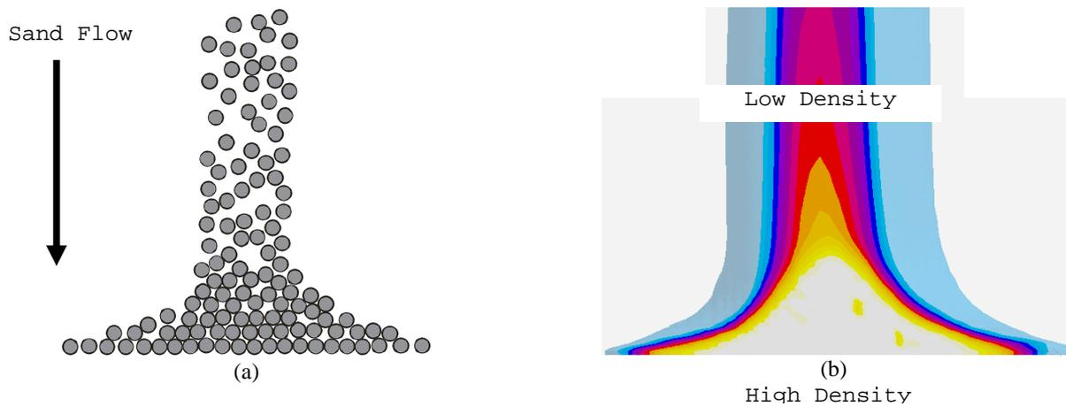
**Fig. 1. Explanatory sphere model (a) and 3D simulation (b) showing sand compaction.**
