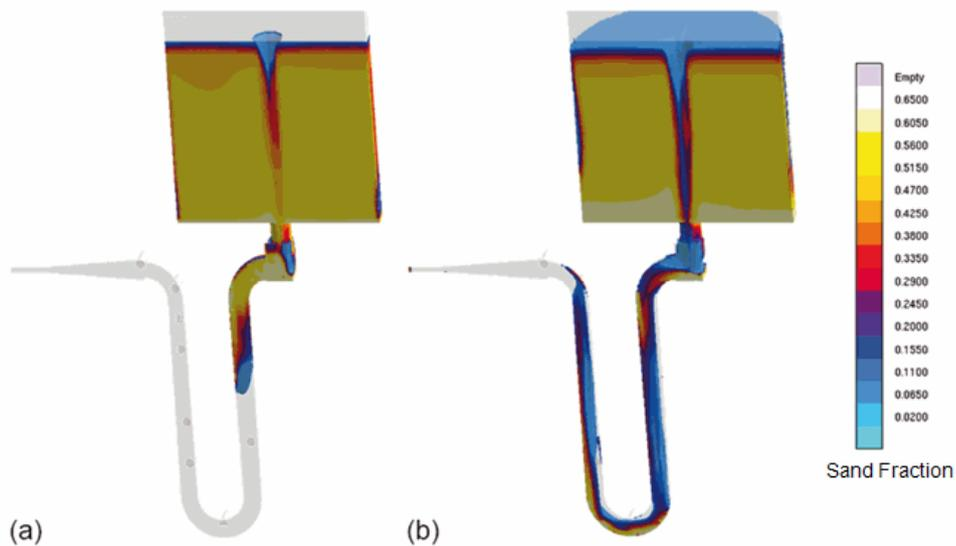
**Fig. 2. Core shooting simulation with simplified hopper at two points in time (a) early in filling and (b) later in filling. In both instances the formation of an area of low sand fraction can be seen in the center of the hopper.**
