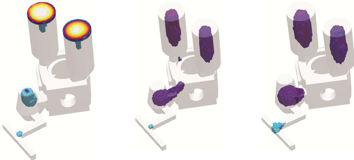
*Fig. 9: Predicted porosity and “critically fed regions” results for the optimized layout (left) and a more robust situation with a slightly larger riser.*
