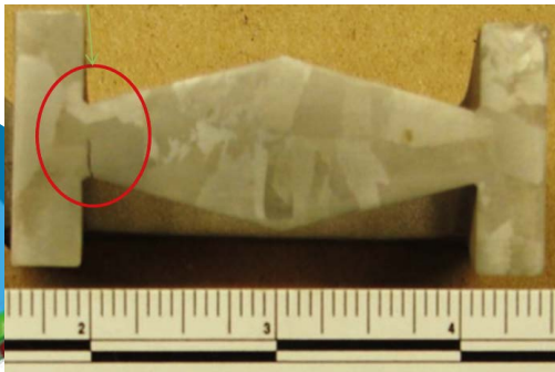
Cracks in the component due to excessive stresses during cooling
