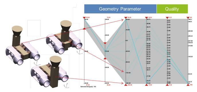
Parallel Coordinates Diagram: Evaluation of different geometries on the selected quality criterion (porosity) in a Design of Experiments
