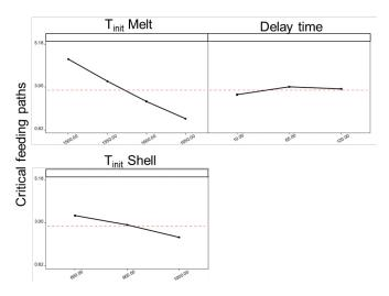
Main Effects Diagram: Influence of process parameters on the feeding behavior in the component
