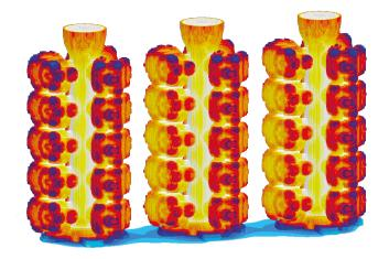
Radiation between heated shell molds and with the environment
