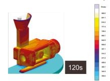
Cooling of the shell mold for different holding times
