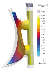
Distortion of the component after shake-out and cooling (magnified representation)
