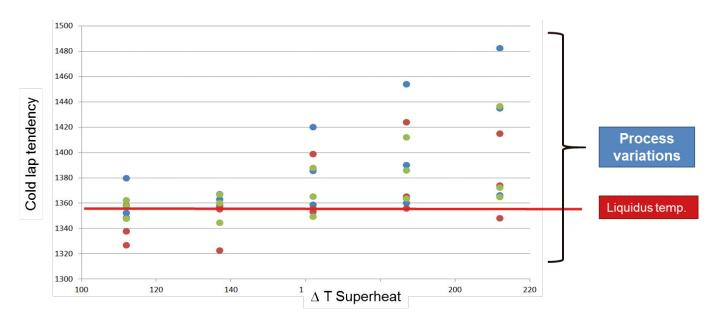
Determination of the risk for cold shuts as a function of process variables and fluctuations
