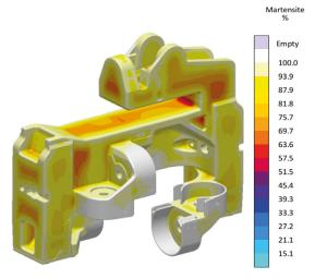
Heat treatment of cast steel: Martensite distribution after quenching and tempering
