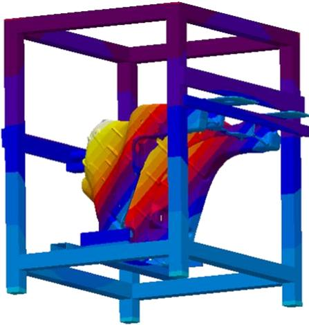
Fig. 4: Fully automatic determination of contact locations between component and frame at any time during heat treatment.
